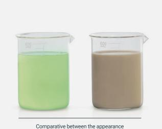
of the Folia and the oil-based fluid after machining.
